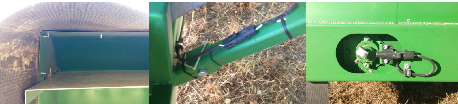
IMAGES (L-R) (1) Looking up the shroud at the end of the deck. (2) Designed with ease of access in mind, all electrics have plugs so the deck can be easily removed. (3) Speed sensor on the conveyor belt.
